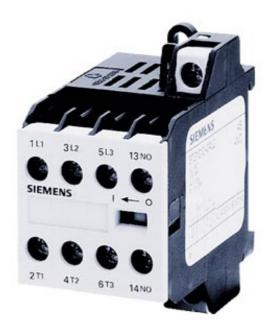
CONTACTOR SCREW TERMINALS, 3NO+1NC FOR SNAPPING ONTO STANDARD MOUNTING RAIL AC OPERATION AC 230V,45...450HZ
