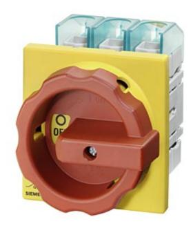
MAIN/EMERG. STOP SWITCH 3-POLE IU=100, P/AC-23A AT 400V=37KW FRONT MOUNTING FOUR-HOLE MOUNTING ROTARY ACTUATOR RED/YELLOW (EMERG. STOP)
