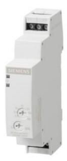
TIMING RELAY, SOLID-STATE, OFF-DELAY, W/O AUX.VOLTAGE, 1 CO CONTACT 7 TIME SETTING RANGES 0.05S...100S, 24-240V AC/DC, WITH LED, SCREW TERMINAL
