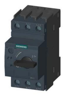
CIRCUIT-BREAKER SZ S00, FOR MOTOR PROTECTION, CLASS 10, A-RELEASE 0.11...0.16A, N-RELEASE2.1A SCREW CONNECTION, STANDARD SW. CAPACITY
