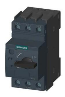
CIRCUIT-BREAKER SZ S00, FOR MOTOR PROTECTION, CLASS 10, A-REL. 0.9...1.25A, N-RELEASE16A, SCREW CONNECTION, STANDARD SW. CAPACITY
