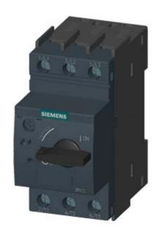
CIRCUIT-BREAKER SZ S00, FOR MOTOR PROTECTION, CLASS 10, A-RELEASE 7...10A, N-RELEASE 130A, SCREW CONNECTION, STANDARD SW. CAPACITY
