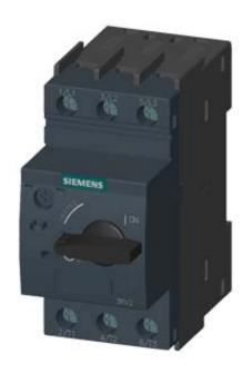
CIRCUIT-BREAKER SZ S00, FOR MOTOR PROTECTION, CLASS 10, A-RELEASE 3.5...5A, N-RELEASE 65A, SCREW CONNECTION, STANDARD SW. CAPACITY
