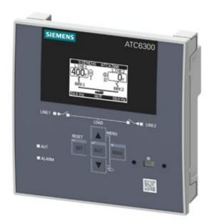
SENTRON 3KC ATC6300; LCD; 144x144 mm; Transfer control device for control of MCCB, ACB, LBS; for load transfer between main and standby power supply Control panel instrument; Un 100...240 V AC 50/60 Hz, 110...250 V DC; Un 12...24 V DC Rated voltage Ue: 100...480 V AC 50/60 Hz; screw terminal connection Expandable by maximum 2 additional modules
