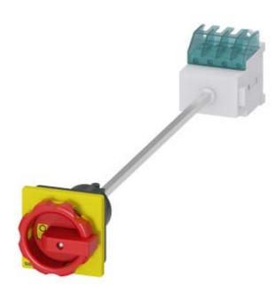
SENTRON, Switch disconnector 3LD, emergency switching-off switch, 3- pole, lu: 16 A, operating power / at AC-23 A 400 V: 7.5 kW, floor mounting with door coupling, rotary operating mechanism, Red / yellow, 4-hole mounting of the handle
