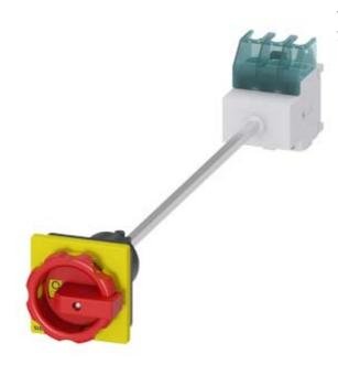
SENTRON, Switch disconnector 3LD, emergency switching-off switch, 3- pole, lu: 25 A, operating power / at AC-23 A 400 V: 9.5 kW, floor mounting with door coupling, rotary operating mechanism, Red / yellow, 4-hole mounting of the handle
