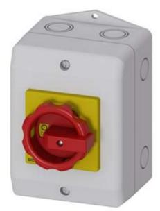
SENTRON, Switch disconnector 3LD, emergency switching-off switch, 3- pole, lu: 32 A, operating power / at AC-23 A 400 V: 11.5 kW, molded-plastic encapsulation for metric cable gland, rotary operating mechanism, red/yellow
