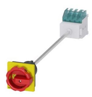
SENTRON, Switch disconnector 3LD, emergency switching-off switch, 4- pole, lu: 16 A, operating power / at AC-23 A 400 V: 7.5 kW, floor mounting with door coupling, rotary operating mechanism, Red / yellow, 4-hole mounting of the handle
