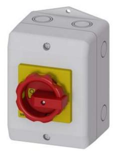
SENTRON, Switch disconnector 3LD, emergency switching-off switch, 4- pole, 16 A, operating power at AC-23 A at 400 V: 7.5 kW, molded-plastic encapsulation for metric cable gland, rotary operating mechanism, red/yellow
