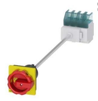
SENTRON, Switch disconnector 3LD, emergency switching-off switch, 4- pole, Iu: 32 A, operating power / at AC-23 A 400 V: 11.5 kW, floor mounting with door coupling, rotary operating mechanism, Red / yellow, 4-hole mounting of the handle
