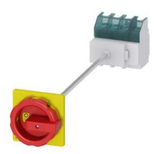
SENTRON, Switch disconnector 3LD, emergency switching-off switch, 4- pole, lu: 63 A, operating power / at AC-23 A 400 V: 22 kW, floor mounting with door coupling, rotary operating mechanism, Red / yellow, 4-hole mounting of the handle
