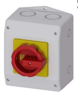
SENTRON, Switch disconnector 3LD, emergency switching-off switch, 3- pole, lu: 63 A, operating power / at AC-23 A 400 V: 22 kW, Molded plastic encapsulation for metric cable gland, rotary operating mechanism, red/yellow
