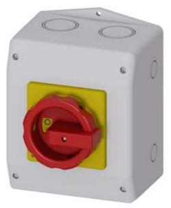
SENTRON, Switch disconnector 3LD, emergency switching-off switch, 4- pole, 63 A, operating power at AC-23 A at 400 V: 22 kW, molded-plastic encapsulation for metric cable gland, rotary operating mechanism, red/yellow
