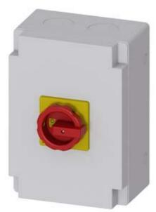
SENTRON, Switch disconnector 3LD, emergency switching-off switch, 3- pole, lu: 125 A, operating power / at AC-23 A 400 V: 45 kW, Molded plastic encapsulation for metric cable gland, rotary operating mechanism, red/yellow
