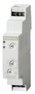
Timing relay, electronic Multifunction 1 change-over contact, 7 functions 7 time ranges 0.05 s ... 100 h 12-240 V AC/DC with LED, Screw terminal
