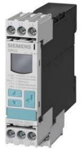
Digital monitoring relay for 3-phase voltage with N-conductor Phase sequence can be activated Phase failure 3 x 90 to 400 V 50 to 60 Hz AC Undervoltage and overvoltage 90-400 V Hysteresis 1-20 V 0-20 s each for Umin and Umax 1 CO for Umin 1 CO for Umax screw terminal Successor product for 3UG3042-1BP50
