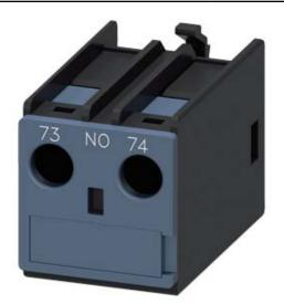
AUX.SWITCH BLOCK,FRONT,1NO, CURR.PATH: 1NO, CONN. F. ABOVE, F. CONT. RELAYS A. MOTOR CONT., 3RT2 SCREW TERMINAL 73 / 74
